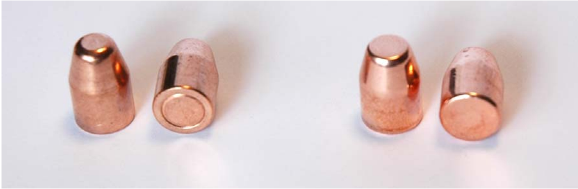
Figure 3. TMJ bullets: Hornady encapsulated (left), West Coast plated (right).
