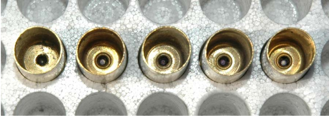
Figure 4. Spent 9mm cases (left to right): WinClean , W231, WST, Clays, Titegroup
