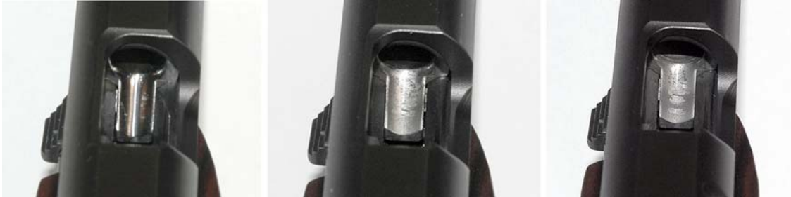
Figure 5. Left to right: clean pistol, pistol after 50 rounds of Winclean, pistol after 50 rounds of Titegroup handload
